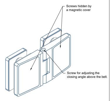
\*See specification Lifting Hinge [DD.0120] Glass to Glass -180° with seal
